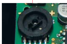
Potentiometer for field settings
