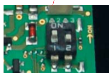
DIP switch for direction detection and cross traffic masking
